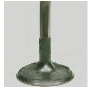
Picture E - Intake valve after P.i. treatment
